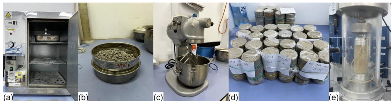
Fig. 3 Test methodology: (a) Drying of sand and PG for 24 hours; (b) Sieving of PG; (c) Mixing of materials; (d) Curing for 3, 7, 14, and 28 days; (e) UCS testing.
